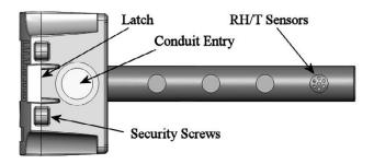
Drill or punch a 1-1/8" or 1-1/4" hole in the duct at the preferred location and insert the probe into the hole to mark the enclosure mounting holes. Remove the unit and drill the four mounting holes. Clean all drilled holes of debris before mounting the device.
