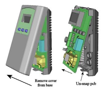
After the base is screwed to an electrical box or the wall using the appropriate holes, pull the wires through the wiring hole in the center of the pcb and then reinstall it in the enclosure base. Ensure the pcb is snapped into the base securely and correctly.
