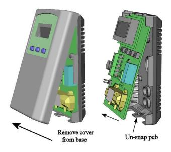
After the base is screwed to an electrical box or the wall using the appropriate holes, pull the wires through the wiring hole in the center of the pcb and then reinstall it in the enclosure base. Ensure the pcb is snapped into the base securely and correctly.
