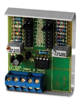
The RTI converts a 3-wire resistance signal to an analog output by using current loop power (two wire). The RTI is reverse polarity protected and offers linear tracking of a 3-wire resistance input against the standard output signal of a 4-20mA (current source). The RTI is small in size and self-powered. These features lends its use to remote mounting for feedback signals from a valve or damper motor indicating its position.
