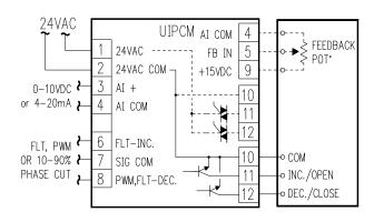
The UIPCM-DC uses two open collector NPN transistors to switch the common in and out, in either PWM or tri-state floating applications.
