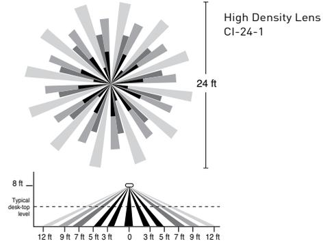
Coverage shown is maximum and represents coverage for half-step walking motion. Under ideal conditions, with no barriers or obstacles, coverage for half-step walking motion can reach up to 1200 ft<sup>2</sup> using the Extended Range lens and up to 500 ft<sup>2</sup> using the High Density lens. For typical desktop level of activity, coverage can reach up to 300 ft<sup>2</sup> using the High Density lens.
