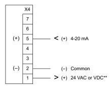
4-20 mA, 2-wire loop-powered sensor/transmitter
