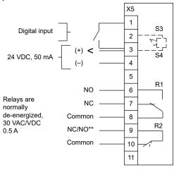
S3 = Built-in horn S4 = Switched output
