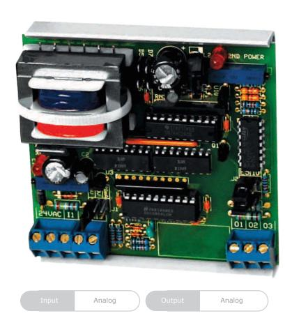
The AIM1 optically isolates an analog voltage or current input signal from its corresponding output signal. The factory calibrated output is linear and proportional (1:1 ratio) to the input signal. The AIM1 will accept a 0 to 5 VDC, 0 to 10 VDC, or 0 to 20 mA input span and output any one of those same ranges. It requires one external 24 VAC isolation transformer for power and has an onboard 24 VAC isolation transformer to supply the isolated output.
