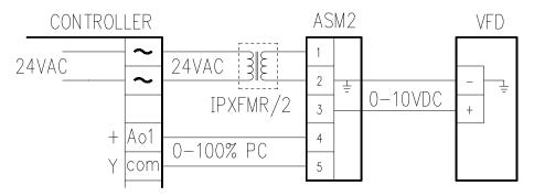
The ASM2/10V converts STAEFA's phase cut signal (0 to 100%) to a 0 to 10V DC output signal to drive a VFD. The ASM2's phase cut input is optically isolated configured to accept the phase cut (+) & (Y) signal, the output signal is referenced to terminal 2 of the 24V AC input which should be transformer isolated from the 24V AC powering the controller to avoid ground loop and/or noise problems generated by the VFD.
