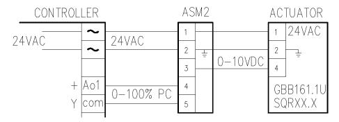
The ASM2/10V converts STAEFA's phase cut signal (0 to 100%) to a 0 to 10V DC output signal to drive Landis or Belimo damper actuators. The ASM2's phase cut input is optically isolated configured to accept the phase cut (+) & (Y) signal, the output signal is referenced to terminal 2 of the 24V AC/DC input.
