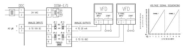
The DISM-E/2/SEQ is factory configured for sequencing operation. For sequencing operation, connect control signal to ch 1 (IN1+/-), select input type Jp1, verify parallel jumper in made, select output action (Jp3,4 D/R) for each output, and output signal type (V DC or mA) for each output. The on-board isolation transformer provides isolation between the two VFDs and the voltage or current output of the DDC controller.
