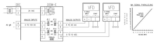
The DISM-E/2/SEL can be field configured by jumpering the parallel jumper for parallel output operation (standard), For parallel operation, connect control signal to ch 1 (IN1+/-), select input type Jp1, select parallel jumper, select output action (Jp3,4 D/R) for each output, and output signal type (V DC or mA) for each output. The on-board isolation transformer provides isolation between the two VFDs and the voltage or current output of the DDC controller.
