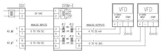
The DISM-E/2/SEL can convert two 0 to 10V DC or 4 to 20mA signals to two 4 to 20mA or 0 to 10V DC output signals. The output signals are isolated from each other and from the two input signals. These isolated signals can be used to drive Variable Frequency Drives, valve or damper actuators. The on-board isolation transformer provides three independent power supplies to power the input section and both output sections avoiding any ground loop potentials.
