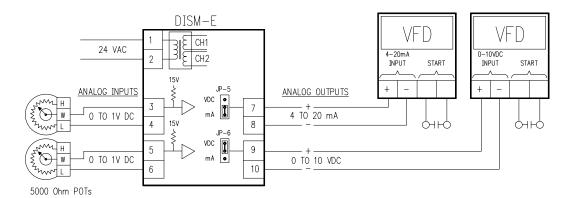
The DISM-E/P2 is factory configured for two 5000 ohm potentiometer inputs to provide a 0 to 100% control of two 4 to 20mA or 0 to 10V DC output signals. The output signals are isolated from each other and from the two input signals. These isolated signals can be used to drive Variable Frequency Drives, valve or damper actuators. The on-board isolation transformer provides three independent power supplies to power the input section and both output sections avoiding any ground loop potentials.
