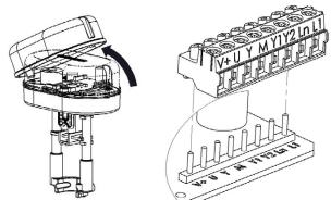
The actuator is equipped with a 8 poles removable terminal block; each pole of the plug is clearly marked and the same label are reported on the electronic board. Before powering up the actuator make sure the plug is properly connected to the board and the label on the plugs and on the board match.
